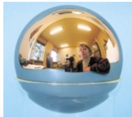
Fig. 1: A “near-perfect” 1 kg Si single crystal. Since “near-perfect”, it acts as a “near-perfect” mirror for IMGC’s Anna Peuto.
