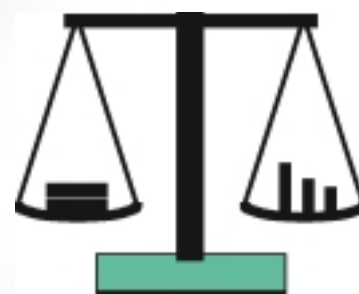
Fig. 2: The balance, used in early chemistry, compares amounts of substance by comparing their weights or masses. From early times, weights (or masses) were compared by a single instrument: the balance. Recognising its status, science gave this measuring process a base (SI) unit, the kg, but science and technology discovered the fact that atoms combine in simple numbers, so chemists cannot use the balance directly to compare amounts of substance. They must divided each mass by “atomic weights” to get what they need. The balance does not take into account the particulate nature of matter.
