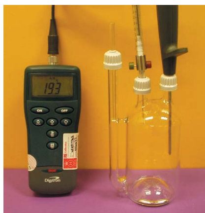
Figure 2. The 'bell-jar' calibration apparatus used to provide a known volume of mercury-saturated air for calibration of the mercury vapour analyser.
